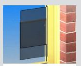
Two panes of glass slide silently past each other within aluminium guides which fit neatly into the perimeter frame.
