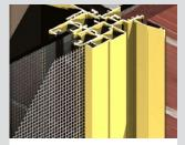
Flyscreen fits neatly into screen receptor channels leaving no unsightly recesses for spiders or dust. Screens are secured with custom nylon spring clips that stop the screens from rattling.
